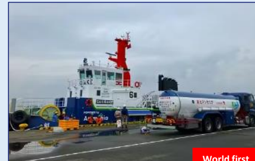
July 2024 Truck to Ship Ammonia Bunkering
